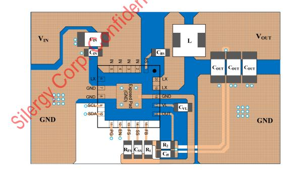
Figure 3. PCB Layout Suggestion
